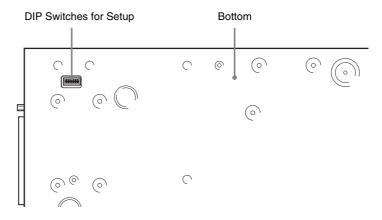
The default factory setting of the DIP switches is as follows.
